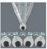
Thanks to the mouth side pivoted by 7.5°, double hexagon geometry and an adjusted application method (placement – screwdriving – turning – turning, etc), even screwdriving challenges allowing a pivoting angle of less than 30° can be solved.
