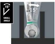
The Joker 6003 ring spanner with its special mouth geometry - a mouth side pivoted by 7.5° and the double hexagon geometry - doubles the placement possibilities when repeatedly turning the wrench 180° around the longitudinal axis. Bolts and screw heads can be "taken" every 15°. The
